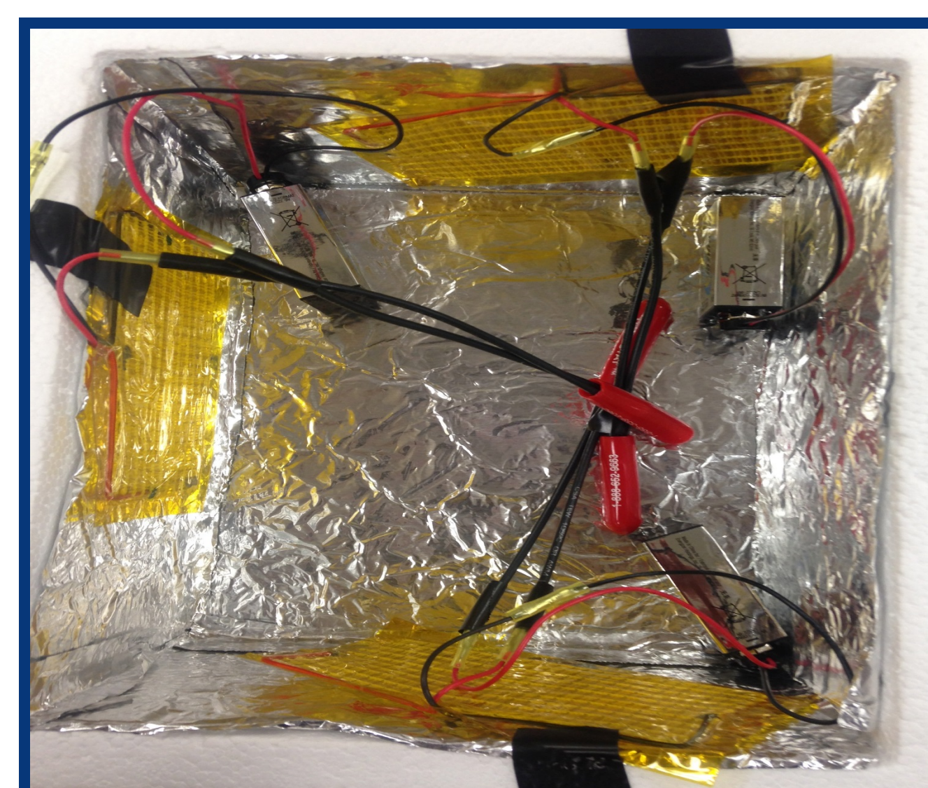
Figure 1. Heating pad, battery, and thermostat configuration used in freezer tests.
