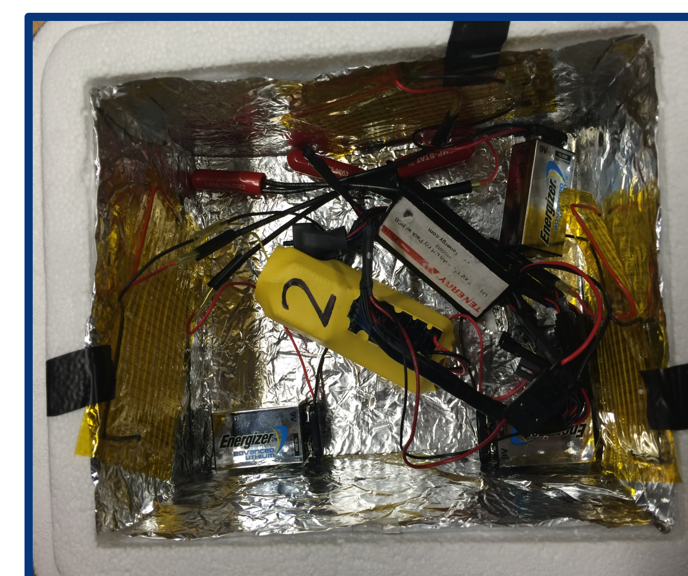
Figure 2. Heating pad, battery, and thermostat configuration used in second balloon flight.
