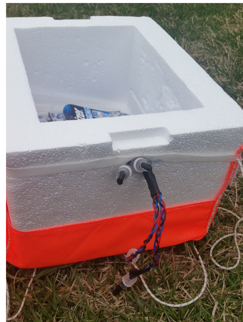
Temperature sensors outside pod
