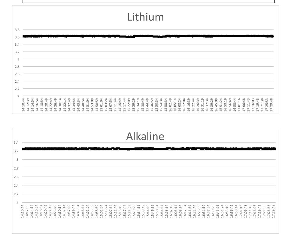
When the balloon reached its highest altitude, both alkaline and lithium had a slightly drop in voltage. At that moment the data also showed the temperature was also at the lowest during the flight, around -45°F.
